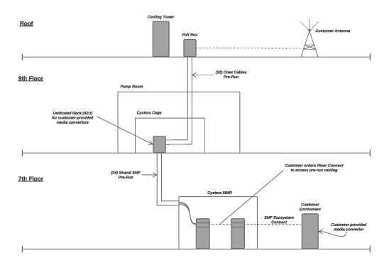
$\underline{\textit{Note}} : \textit{Connections to endpoints on 8th Floor or 4th floor will use existing fiber between all Cyxtera \textit{MMR}'s. \\$
